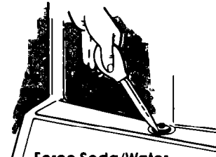
Force Soda/Water Solution Through Drain Cap Openings.
